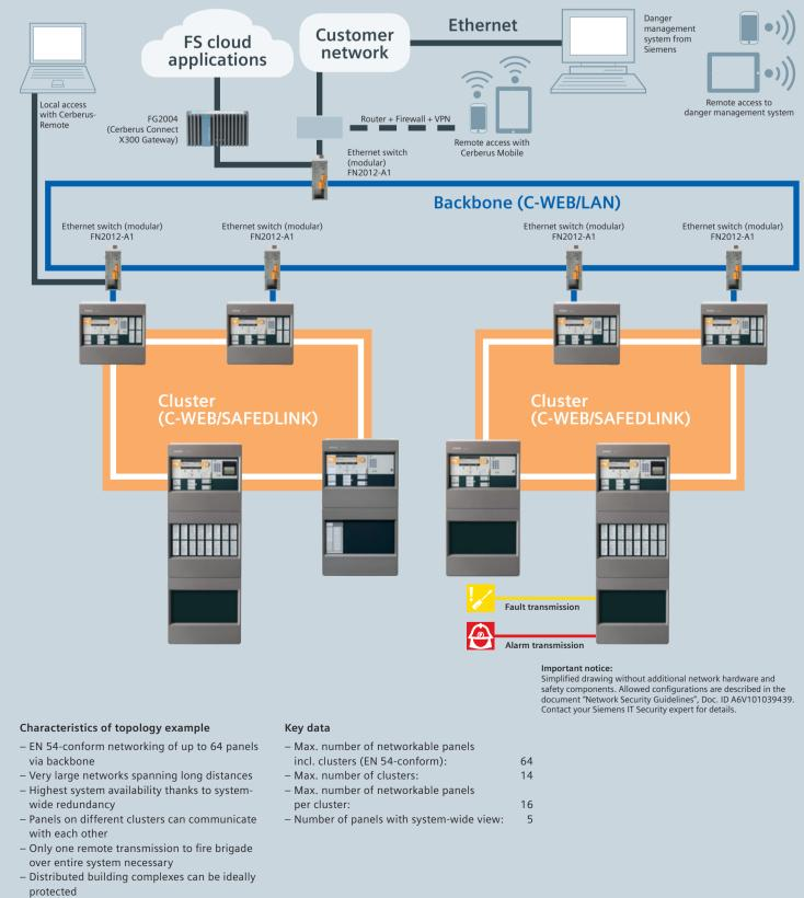
– Backbone is realized with fiber-optic cable
